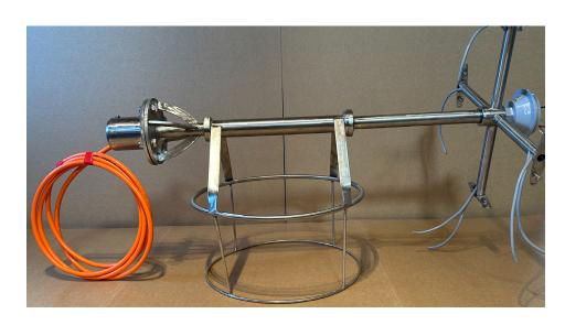
Beacon and LED Lights prewired for final installation at site (licenced electrician required)
