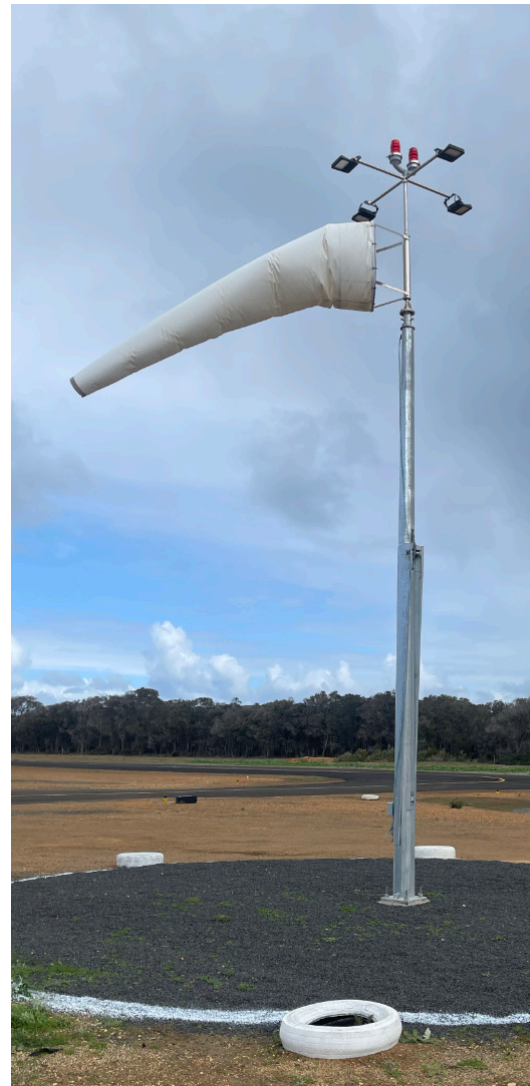
Indicative Installation. IWDI with LEDs and Obstruction Lights mounted on fully SS Dual 900m \varnothing Windsock Frame with CASA Aviation Grade Windsock. IWDI is mounted on 6m Extra Heavy Duty Counter Weighted Galvanised Pole
