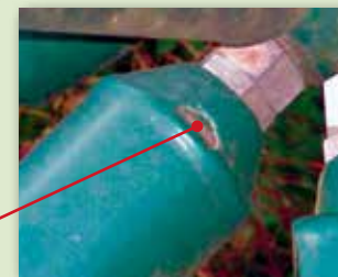
► No under-film corrosion after 12 years.
