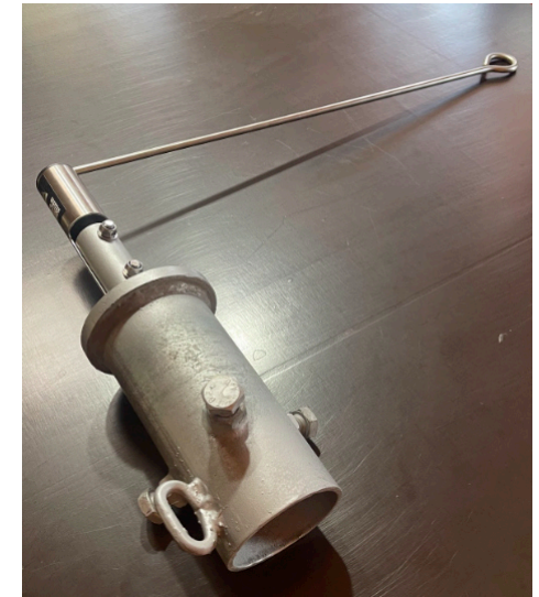
Windsock is clipped via a Bridle Harness into to a SS HD Rotor Arm Pivot mounted on a DN80 Spigot fastened to the top of the pole
